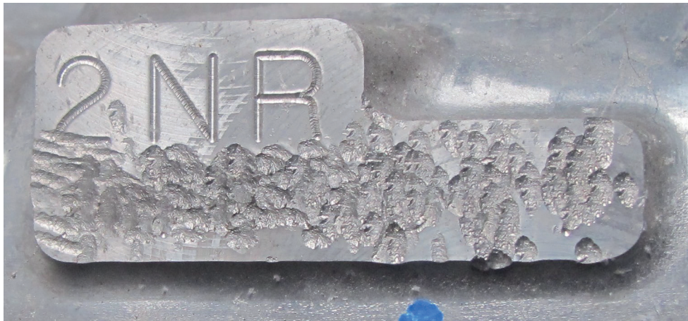
Fig. 1. The method of welding the number field or the relatively deep removal of characters made by chiselling or laser-burning causes irreversible changes and the inability to reveal the removed characters.
