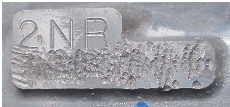
Fig. 4. Number field of the gearbox before testing. Source: own resources.
