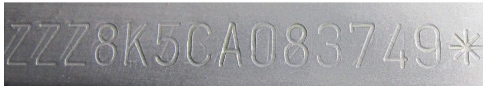
Fig. 3. VIN after etching with Adler II reagent. Source: own resources
