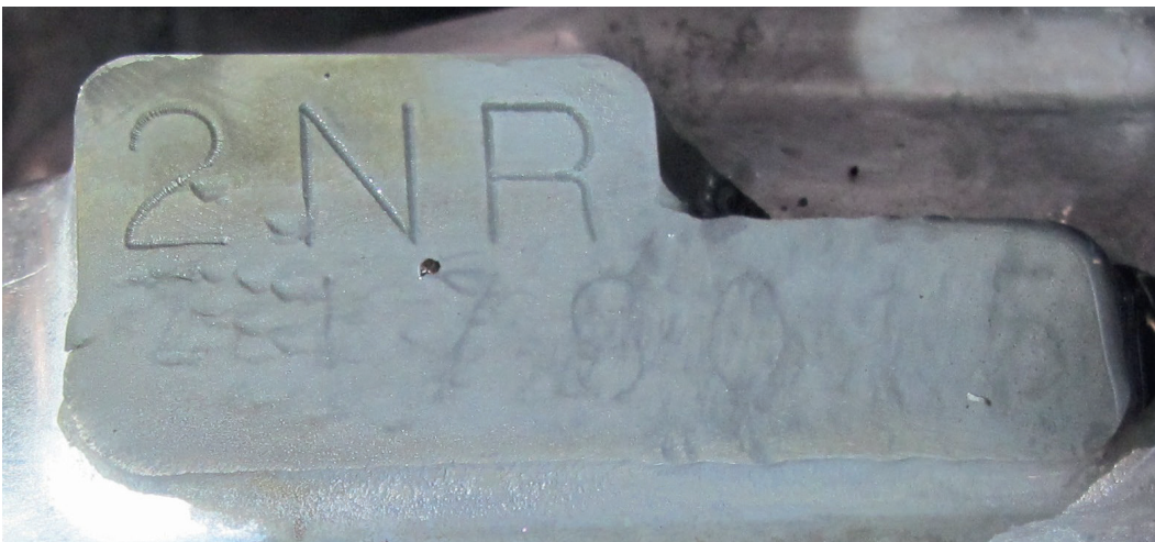
Fig. 6. Number field during etching with Adler II reagent.
