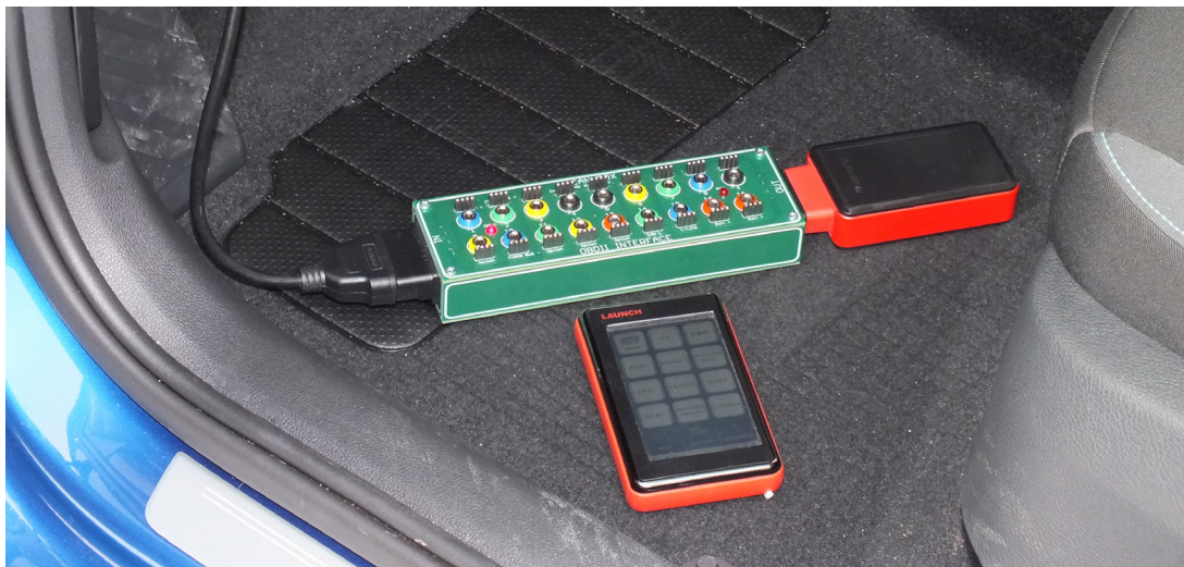
Fig. 7. The practical application of CAN-BOX in a vehicle together with a diagnostic tool
