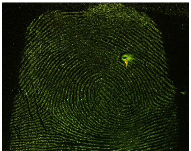
Fig. 34. Fingerprint revealed on a ceramic plate using the NANODAK 40 suspension, registered in blue light of the wavelength of 410 nm, with a yellow filter
