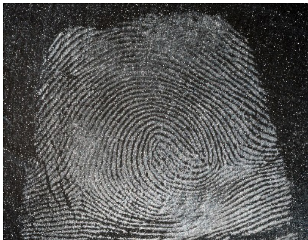
Fig. 41. Fingerprint revealed on a ceramic plate using the NANODAK 1 nanopowder, registered in white light
