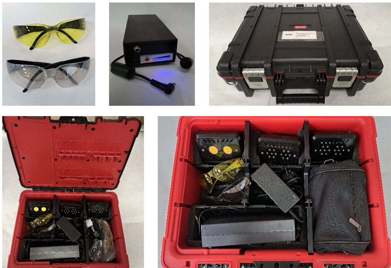
Fig. 4÷9. FA set of LED illuminators with auxiliary equipment
