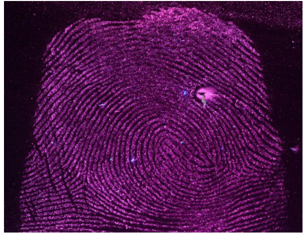
Fig. 32. Fingerprint revealed on a ceramic plate using the NANODAK 40 suspension, registered in UV light of the wavelength of 360 nm, with a colourless filter
