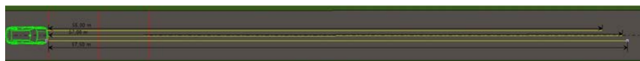
Fig. 10. A light spot range of 10 lx of dipped with brand new headlight covers and used bulbs
