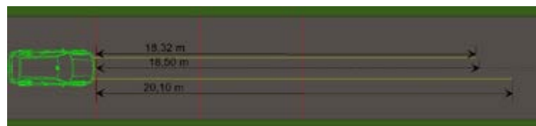
Fig. 9. Light spot range of 10 lx dipped with faded headlight covers and with new, more powerful bulbs
