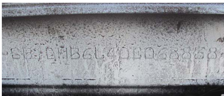
Fig. 4-5. Vehicle number field test using a permanent magnet defectoscope
