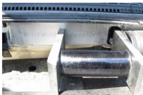
Fig. 4-5. Vehicle number field test using a permanent magnet defectoscope
