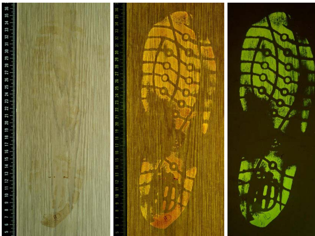
Fig. 12, 13, 14. Blood footwear impression visualised by Acid Yellow 7 visible in white light (left), in fluorescence (middle), and in fluorescence after being transferred from the surface to a gelatin lifter (right)
