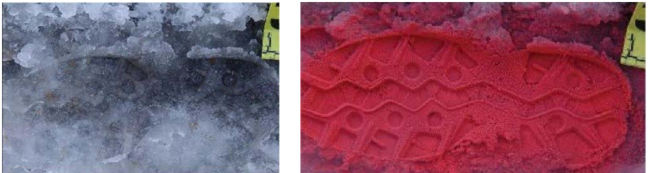
Fig. 10, 11. Three-dimensional snow impression before (left) and after (right) contrasting with Snow Print Wax
