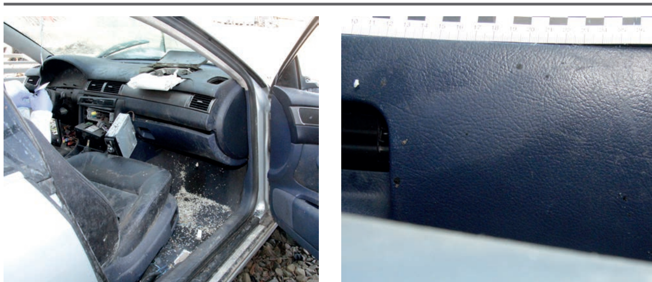
Fig. 8. Interior of the AUDI A6 vehicle tested and a close-up of the scratches found on the surface of the glove compartment door.
