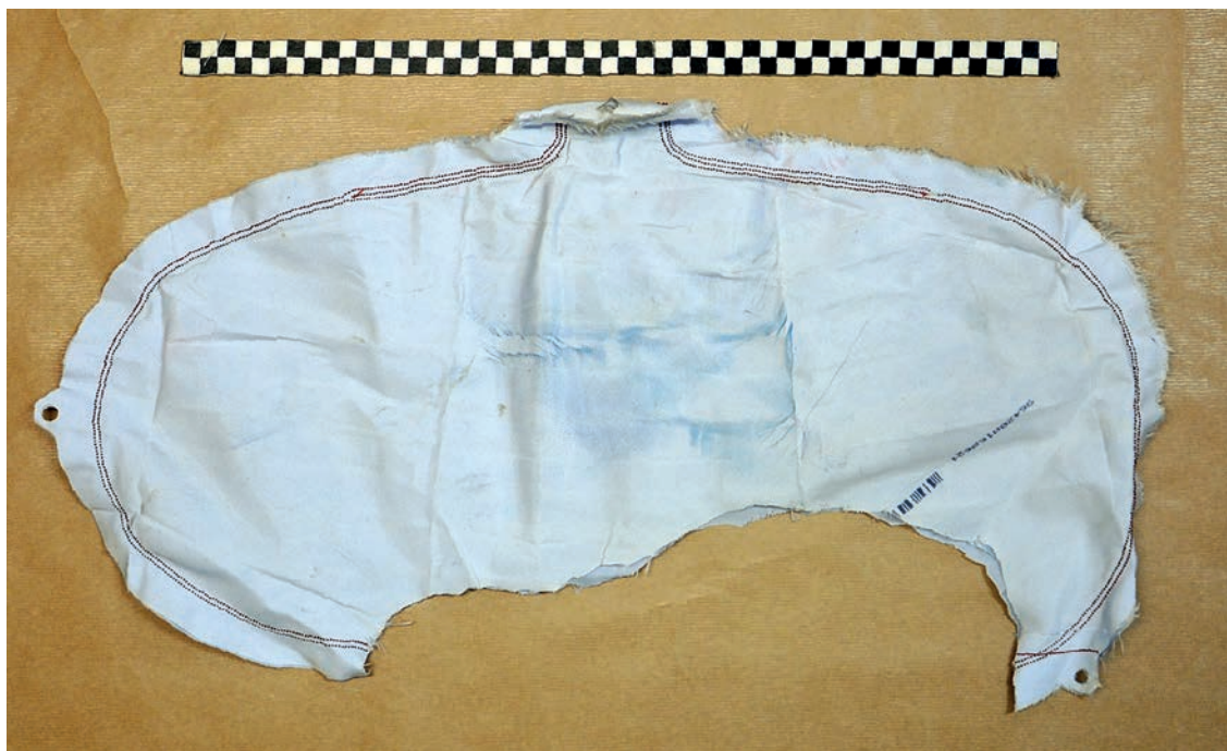
Fig. 6. Deployed driver side airbag with visible marks of a blue substance
