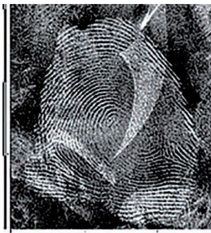
Fig. 20, 21. Fingerprints revealed on the can and scanned with TrasoScan System under 365 nm illumination and using a yellow visual filter.
