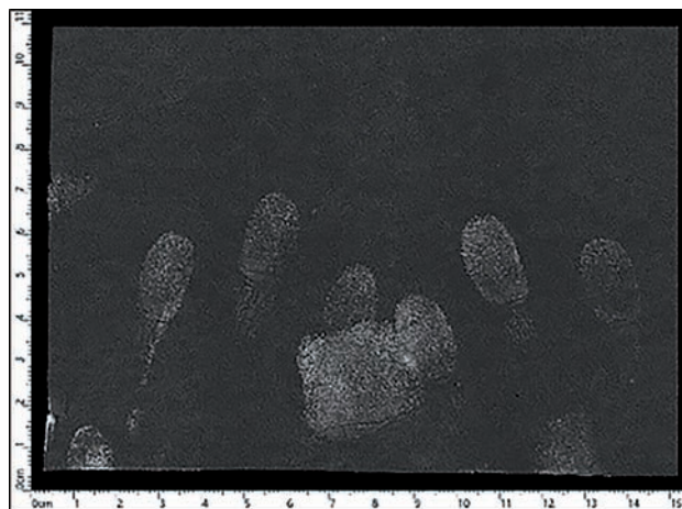
Fig. 2. Fingerprints revealed by the DFO technique and scanned with the TrasoScan System.
