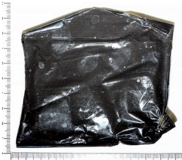
Fig. 7. A black stretch film containing fingerprints revealed with cyanoacrylate fumes, photographed with a digital camera.
