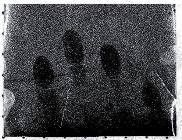
Fig. 11. Gelatin film with the cover removed, containing fingerprints secured in the dust, scanned with TrasoScan System.
