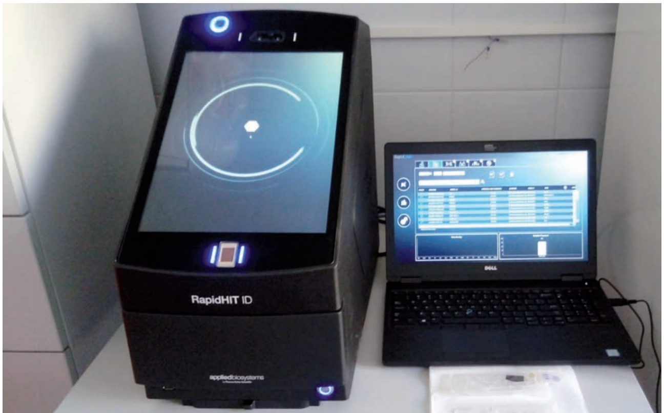
Fig. 2. RapidHIT™ ID with connected to the computer with installed software and disposable cartridges (ACE Sample Cartridge).
