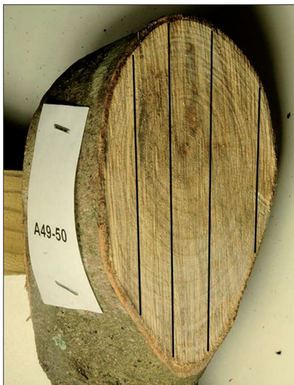
Fig. 5. Type 1 Striation pattern.
