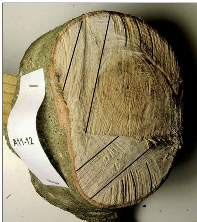
Fig. 7. Type 3 Striation pattern.
