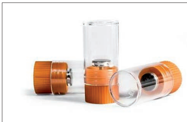
Fig. 26. View of the special stage for SEM studies.
