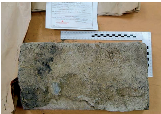
Fig. 2. Evidence material – concrete block, bottom surface with visible mortar.
