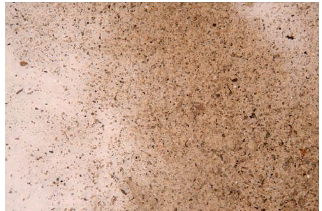
Fig. 23. Shakeout sample designated as MD3 (jeans trousers) (10× magnification).
