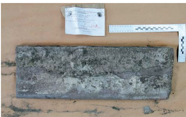
Fig. 4. Comparative material – 3 pieces of concrete blocks, bottom surface with visible mortar; designated as MP1, MP2, MP3.
