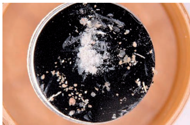
Fig. 27. Exemplary material applied to a stage for SEM studies.
