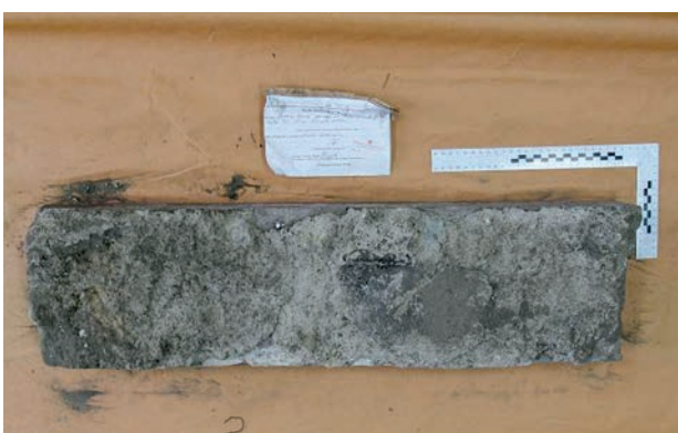
Fig. 2. Evidence material – concrete block, bottom surface with visible mortar.
