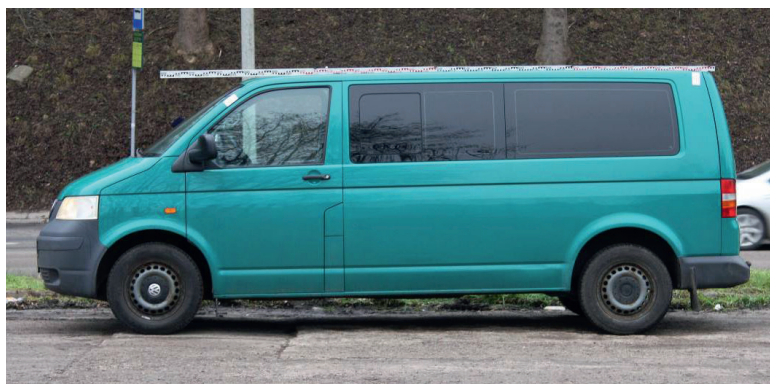
Photograph 2. A photograph with a focal length of 50 mm of a Volkswagen T5 vehicle taken according to the rules, i.e. perpendicular to the side of the vehicle
