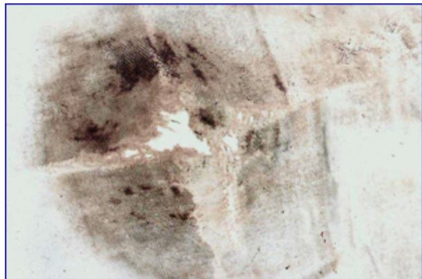
Result of colour reaction of lead with sodium sulfide
